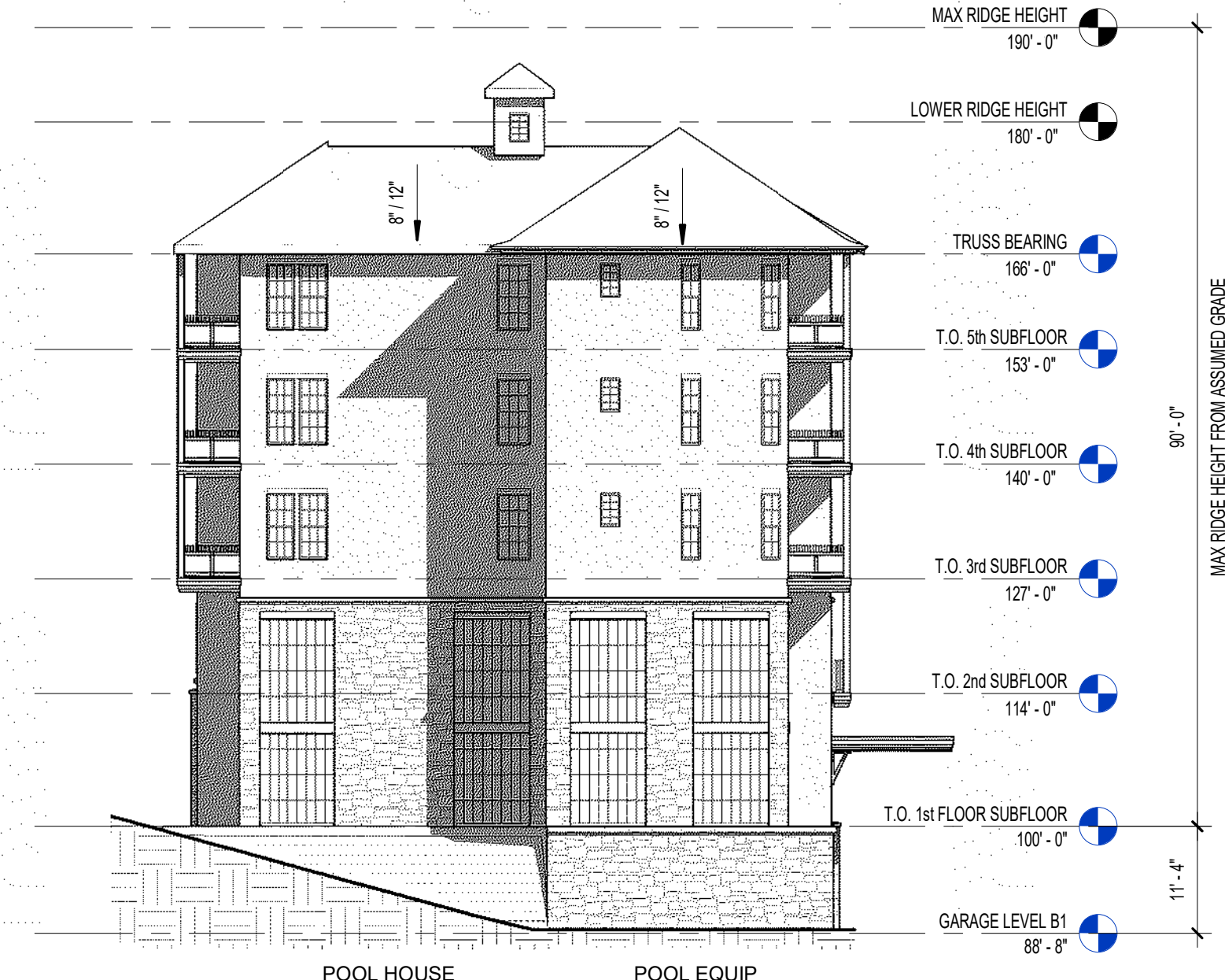
6 SOUTH IL WING ELEVATION 1/16" = 1'-0"
