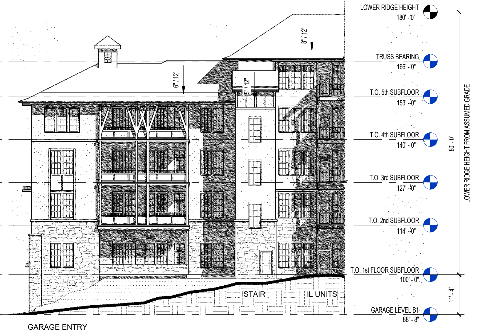
3 NORTHWEST IL WING ELEVATION 1/16" = 1'-0"
